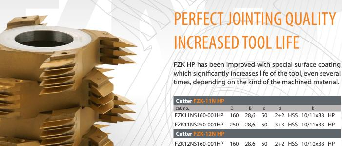
Construction changes in the technological process and blade geometry of the FZK cutters allowed to obtain perfect jointing quality and increased tool life. Quality and life of the blade has been considerably increased by using high quality fast-cutting steel and proper heat treatment which resulted in optimal blade hardness as well as proper small grain steel structure and impact resistance.
